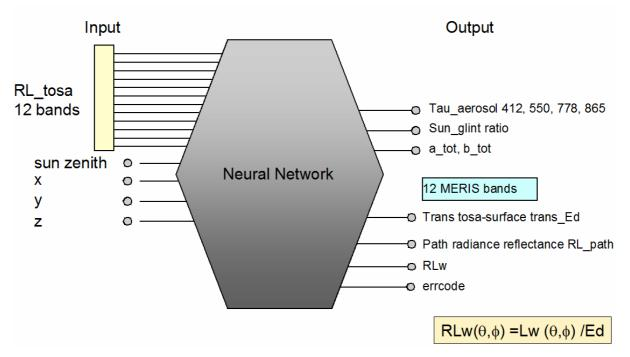
Figure 3: Outline of the neural network to determine the water leaving radiance reflectance RLw.
