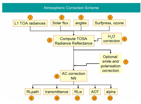
Figure 2: Atmospheric correction scheme
